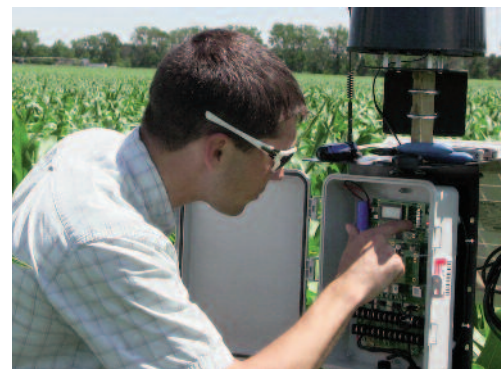
Figure 1. Soil moisture monitoring. This telemetry unit incorporates a tipping bucket rain gauge in addition to soil moisture sensors.
