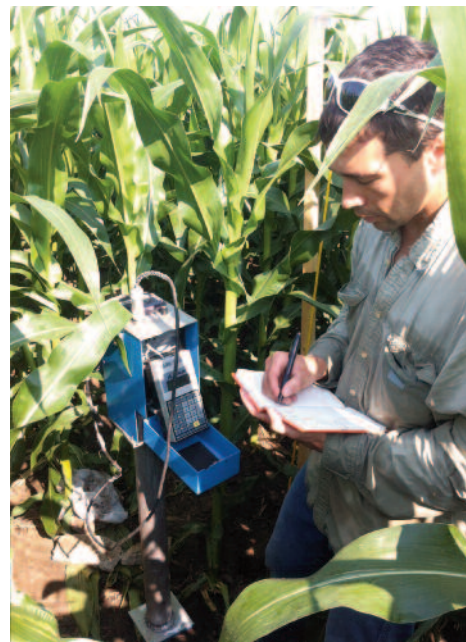
Joshua Stamper uses a Neutron Probe to measure soil moisture in a field with VRI at the Anderson Farm in Belgrade, MN.
